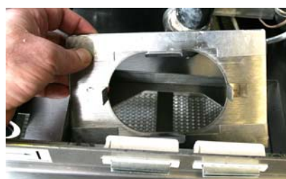
Figure 7: Position the splashguard in the apron, which surrounds the downspout opening on the filter pan lid.
