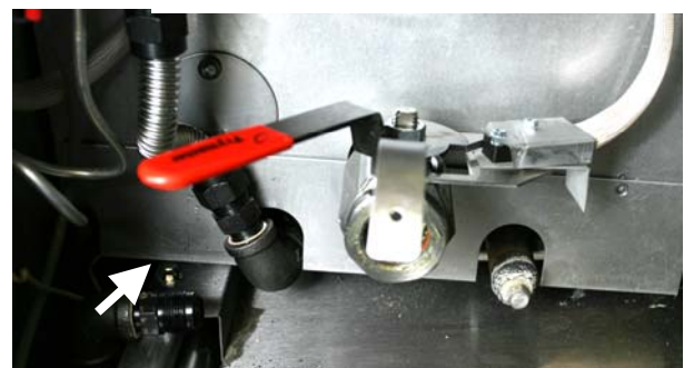
Figure 3: In some models sheet metal screws secure the filter pan lid. Remove the skirt in front of the burner to access the screws.
