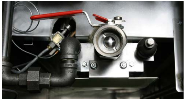
Figure 2A: The bracket is shown attached to the burner manifold and the shield suspended from the studs of the bracket, secured with the provided 1/4-20 nuts (809-0417).
