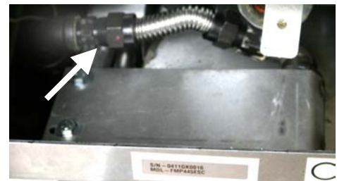
Figure 2: Remove the flexline from the street L, See arrow.
