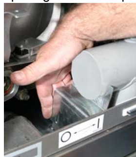
Figure 7: Position the splashguard in the apron, which surrounds the downspout opening on the filter pan lid.
