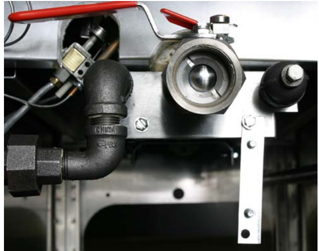
Figure 1A: The bracket (106-5141) is shown partially attached to the burner manifold using existing nuts. The studs, which provide a mounting point for the heat shield, are extended out.
